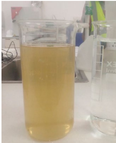
Effluent from Mudor WWTP
